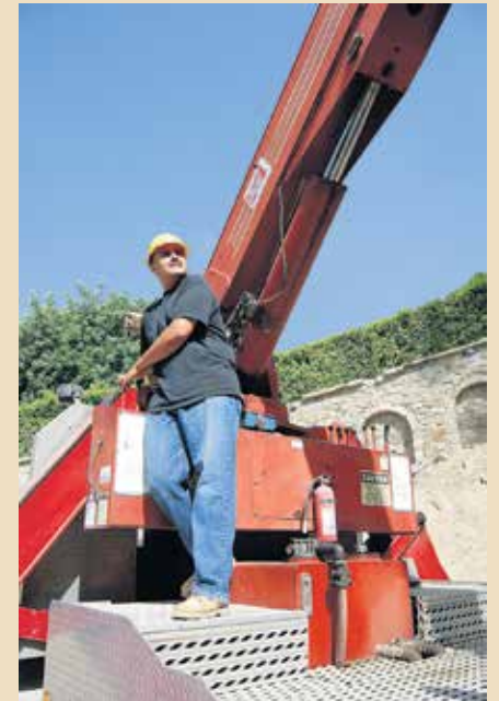
Mobile cranes are often de-rated in order to enable their use by a less qualified operator, ministry says. File photo
