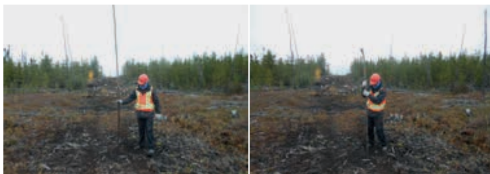
FIGURE 18. The use of a simple soil probe can aid in estimating soil depth and determining drainage structure placement.
