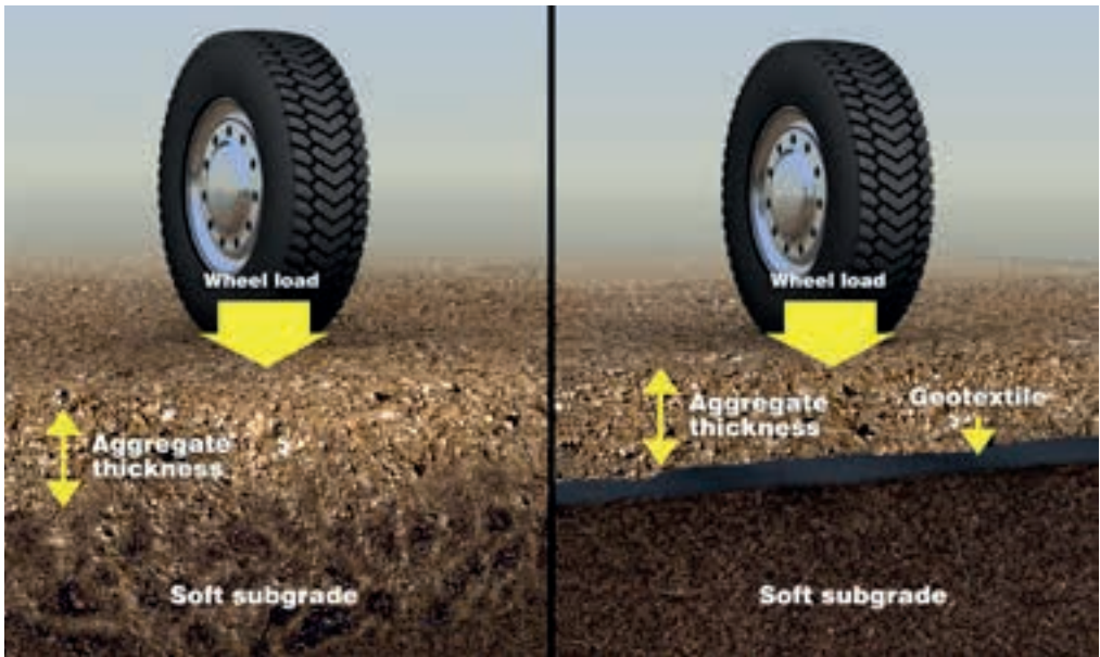
FIGURE 25. Geotextiles can act as a separation layer to minimize bearing failures and reduce aggregate thickness.
