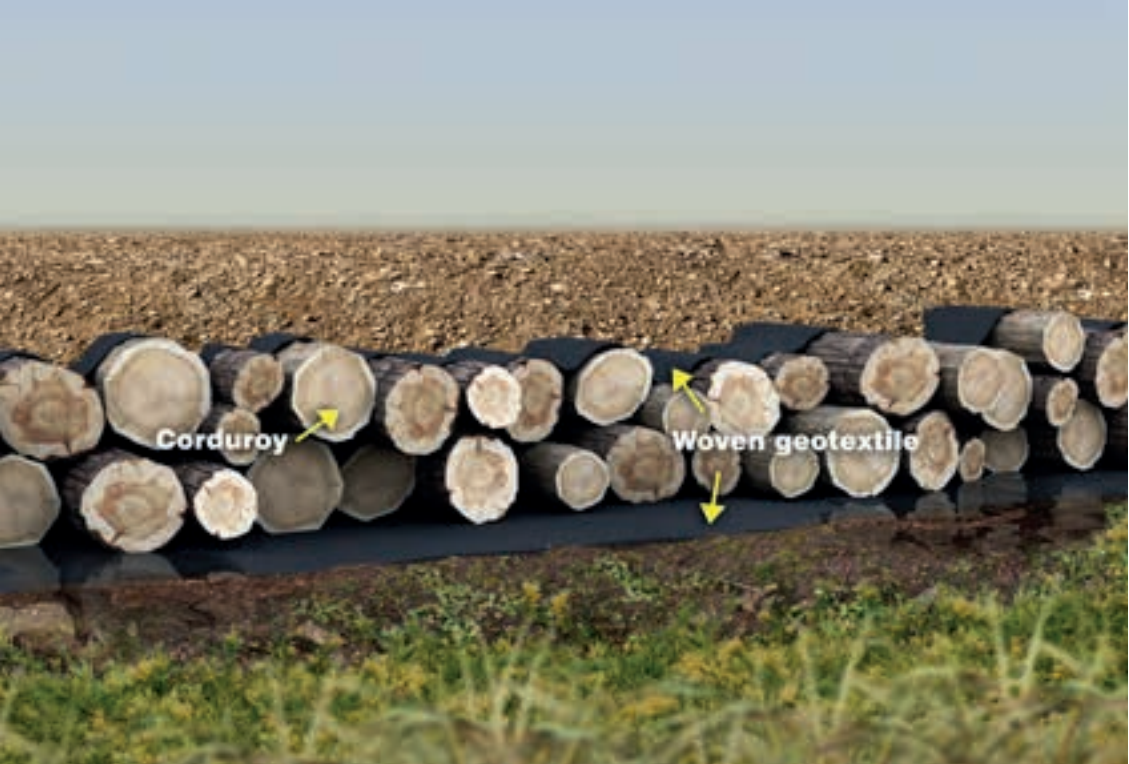
FIGURE 55. Example of a corduroy structure to provide water flow through a road.
