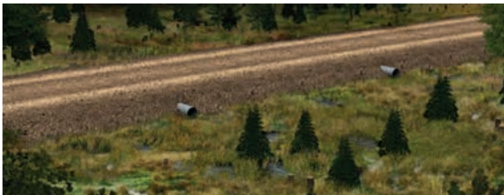
FIGURE 47. To provide for wetland flow in stagnant wetlands, use widely spaced, small-diameter culverts.
