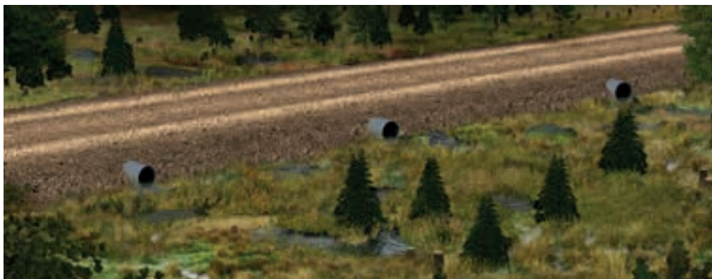
FIGURE 48. To provide for wetland flow in slow lateral-flow wetlands, use mid-sized-diameter culverts.
