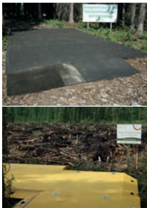
FIGURE 40. Rubberized mat made of recycled rubber tires (top) and a composite plastic mat (bottom). (Photo courtesy of Alberta Environment and Parks.)
