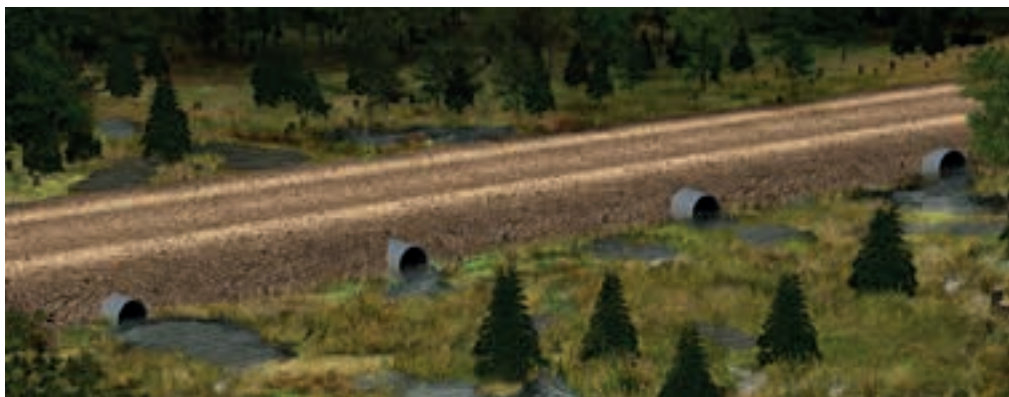
FIGURE 49. To provide for wetland flow in seasonally fluctuating wetlands, use closely spaced, large-diameter culverts.
